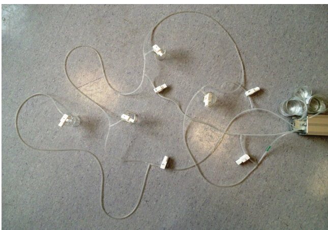
Figure 4. Designed apparatus arrangement for the continuous production of CaP-PDADMAC/PSS nanoparticles
