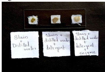
Figure 11. Leaf extract stain removal test
