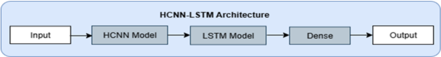
Fig. 3. Architecture of the proposed Hybrid Convolutional Neural Network–Long Short-Term Memory (HCNN-LSTM) model, showing the sequential flow from the embedding layer through the one-dimensional convolutional layer, max-pooling layer, LSTM layer, dropout regularization (rate = 0.5), and final fully connected softmax output layer.
